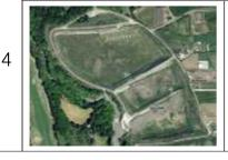
The artificial recharge site was constructed from 2007 to 2011 to secure water resources as well as to control flood. The reservoir volume in the Hancheon stream is about 900,000M3, and there are 10 vadose injection wells of 40-50m depth. During the flood season in 2010, about 2,500,000 ton of water was recharged in the reservoir.
