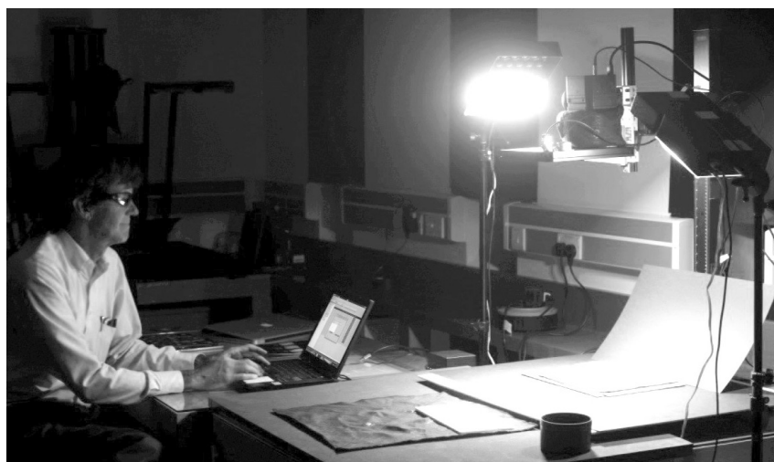
Multispectral imaging with Phase One cameras and integrated Equipoise Imaging narrowband LED illumination in ultraviolet-visible-infrared wavelengths by Michael B. Toth of R.B. Toth Associates LLC.
