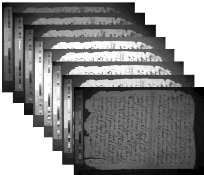
A stack of registered images of the Birmingham Qur'an captured with a 100 megapixel Phase One color camera and Equipoise Imaging narrowband illumination in multiple spectral bands of light from ultraviolet through visible and into infrared bands.
